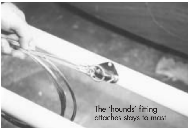
Fitting the masthead
