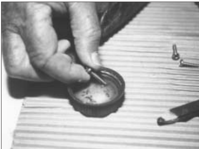
Dip screws in linseed oil or similar but not glue
